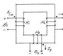
Generalizing the two-winding transformer, additional windings can be used to form multi-winding transformers.
