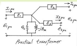
The shunt admittance can be determined by the open-circuit test and the series leakage impedances can be found by the short-circuit test as was done in two-winding transformer.
